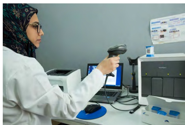
Aya Awade, a laboratory technician at Karantina Tuberculosis Center in Beirut, Lebanon, operates a GeneXpert machine purchased with Global Fund support that increases the center's TB testing capacity by dramatically reducing the time it takes to get a diagnosis. This technology can be repurposed to test for COVID-19 as well. The Global Fund/Sarah Hoibak
